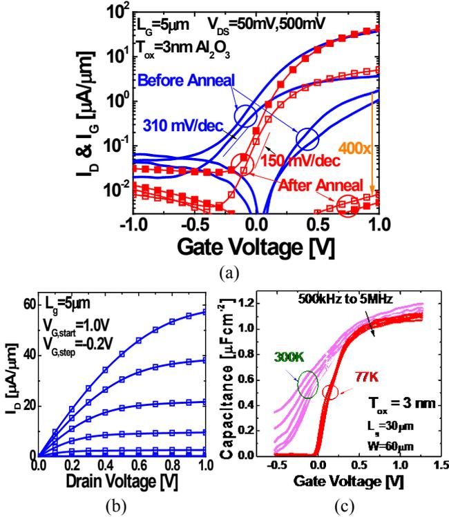
Fig. 2. (a) Transfer characteristics of the  $L_G=5\mu\text{m}$  device. (b) Output characteristics of  $L_G=1\mu\text{m}$  device, showing very good saturation without any effects of impact ionization. (c) Split C-V characteristics at 77K and 300K.
