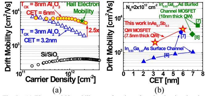
Fig. 3. (a) Electron drift mobility as a function of carrier density showing 2.5x enhancement on scaling oxide thickness. Record high electron mobility of  $5200 \text{ cm}^2/\text{Vs}$  achieved for the device with  $8\text{nm}$  oxide at  $N_s=1.8 \times 10^{12}/\text{cm}^2$ . (b) Electron drift mobility as a function of CET for the thin QW device (CET is obtained from split C-V and it includes semiconductor capacitance).
